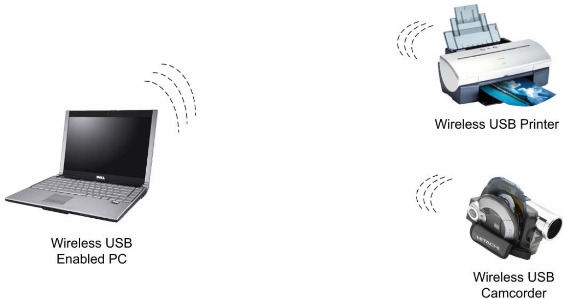
Figure 1: A Wireless USB Host (PC) connected to Natively Wireless Peripherals
